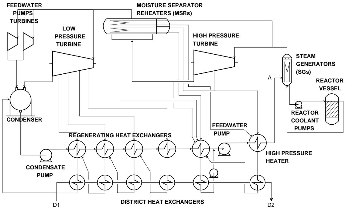
Figure 9: Diagram of NCHP using heat from the regenerating heat exchangers
