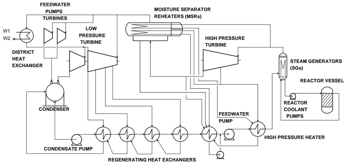
Figure 8: Diagram of NCHP using heat from the bleed steam
