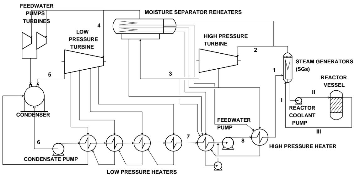
Figure 4: Diagram of the power station without modifications
