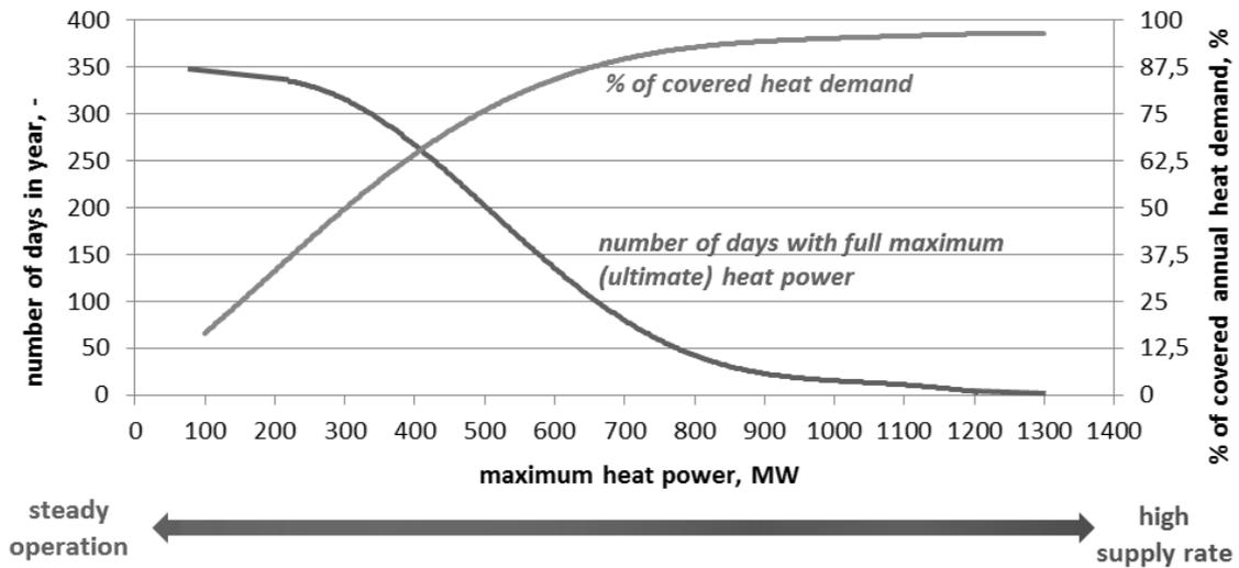
Figure 3: Diagram of heat demand showing assumed load of the heat network
