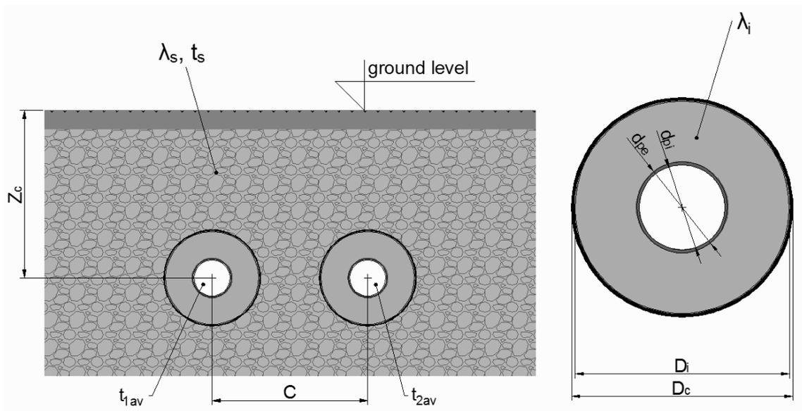
Figure 6: Model of pipeline heat loss calculations
