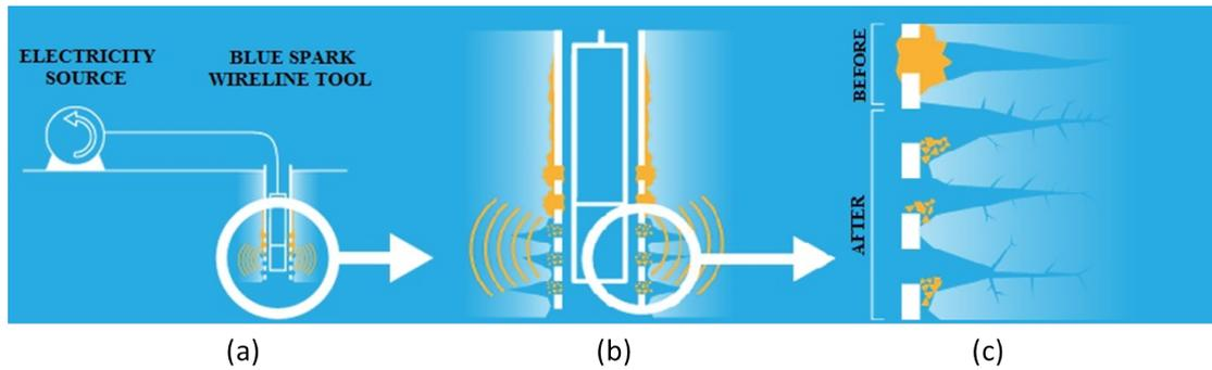
Figure 1: Schematic diagram of an application of pulsed high-voltage discharge technology: (a) Structure of pulsed high-voltage discharge system; (b) Electrohydraulic effect generated by downhole discharge; (c) Dredge oil pipe
