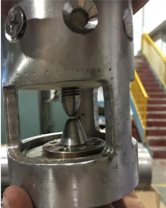
Figure 12: Electrode erosion
