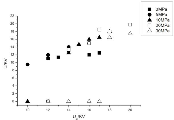
Figure 8: Influence of static pressure on the discharging voltage with water as the discharging medium
