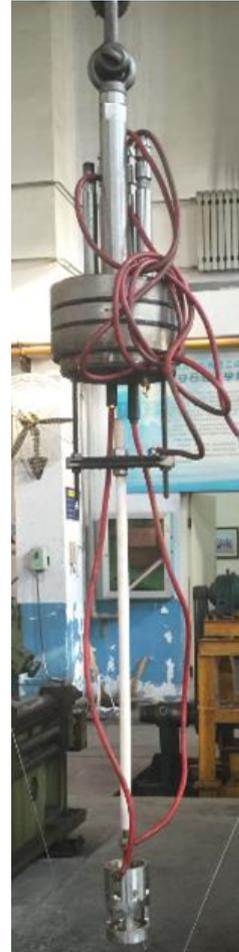
Figure 6: Connection mode of the discharging electrode inside the HPSD
