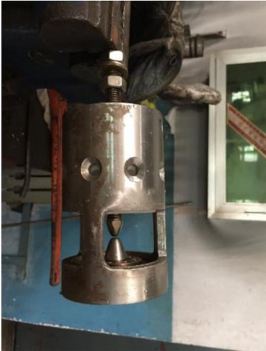
Figure 5: Structure of the discharging electrode
