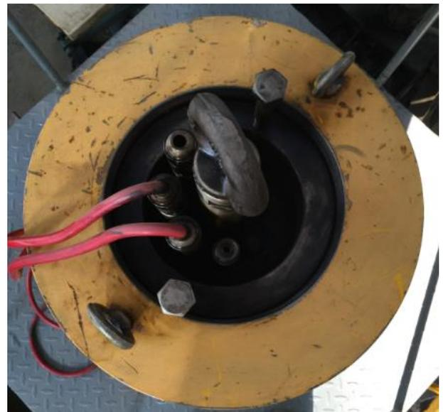
Figure 3: Arrangement of sealed contact pins
