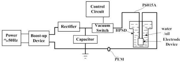
Figure 4: Schematic diagram of the experimental system of pulsed high-voltage discharge
