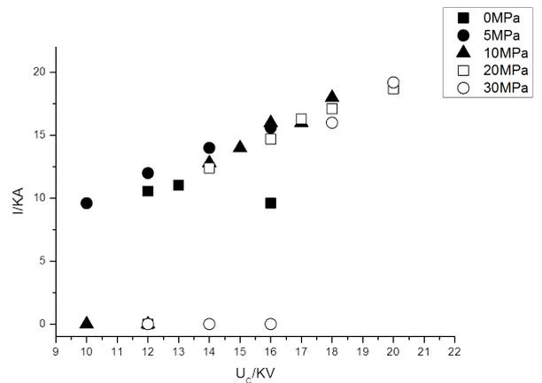
Figure 9: Influence of static pressure on the discharging current with water as the discharging medium
