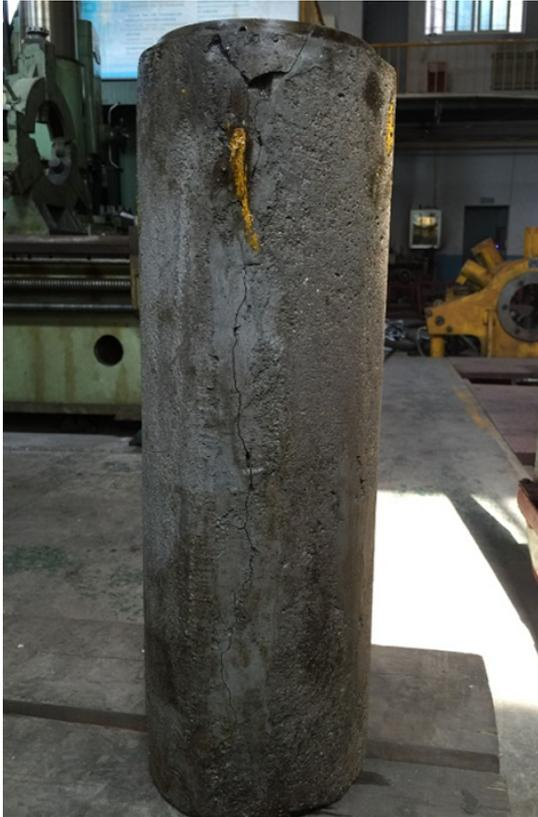
Figure 10: Damaged cement tube at static pressure of 15 MPa
