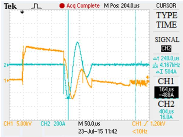
Figure 7: Voltage and current oscillographs under discharging breakdown in water
