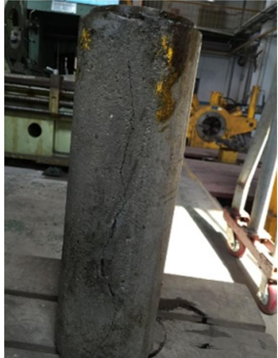
Figure 11: Damage of cement tube at static pressure of 30 MPa
