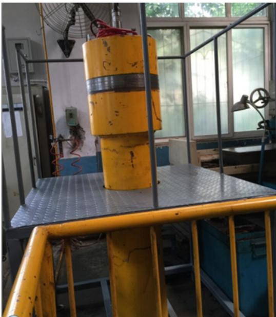
Figure 2: External structure of the high-pressure sealed drum (HPSD)
