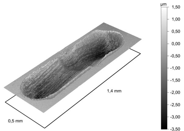
Figure 8: Wear scar on the plate used in the HFRR test
