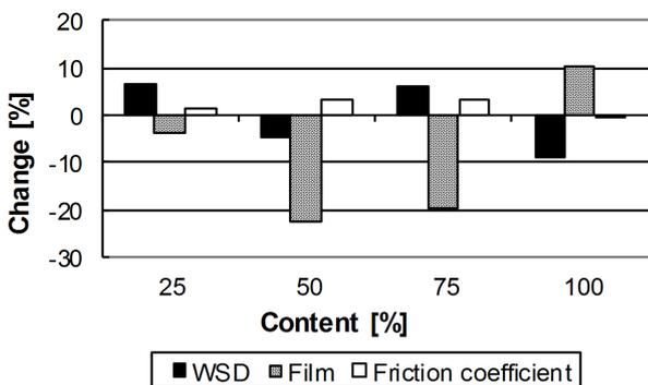
Figure 6: Change in lubricating properties depending on mix1 content in ESSOMARCOL oil
