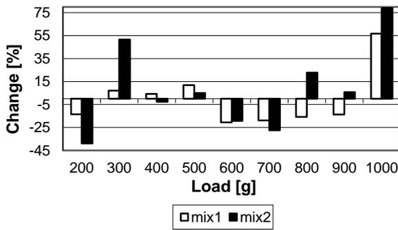
Figure 9:  $R_a$  variation of mix1 and mix2 compared with ESSOMARCOL oil
