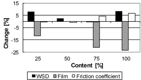
Figure 7: Change in lubricating properties depending on mix2 content in ESSOMARCOL oil
