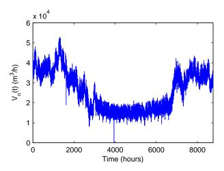
Figure 1: Hourly demand curve in municipal area (flow at standard conditions of 101.325 kPa and 273.15 K).
