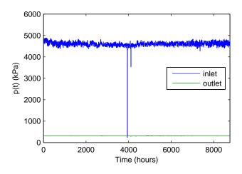
Figure 2: Inlet and outlet pressure profiles (gauge pressure) in Case study I.
