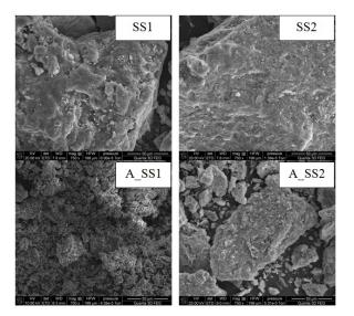
Figure 8: SEM images of raw sewage sludge and obtained ash
