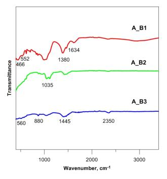
Figure 4: FTIR images of biomass ash
