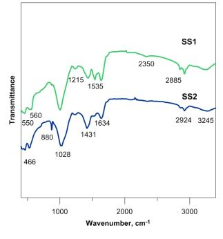
Figure 5: FTIR images of raw sewage sludge
