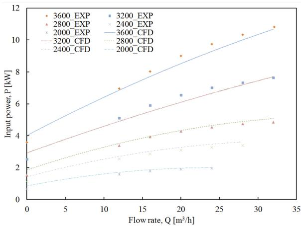
Figure 6:  $P$ - $Q$  curves of experiment and CFD simulation
