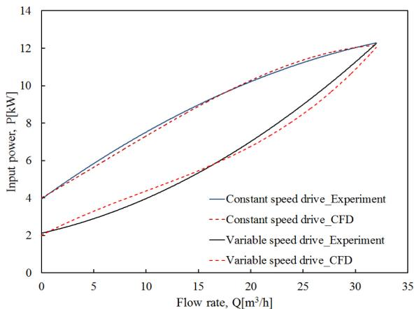
Figure 9: P-Q curves with constant and variable speed drive
