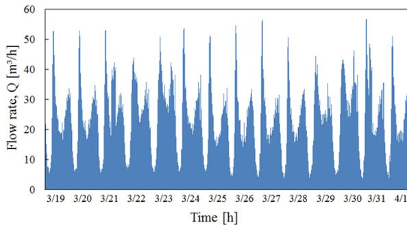
Figure 3: Flow rate pattern of feed water pump
