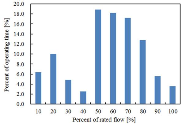
Figure 4: Mean duty cycle of feed water pump
