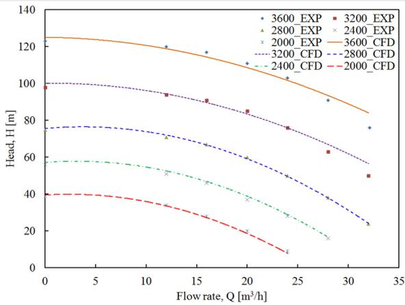
Figure 5:  $H$ - $Q$  curves of experiment and CFD simulation
