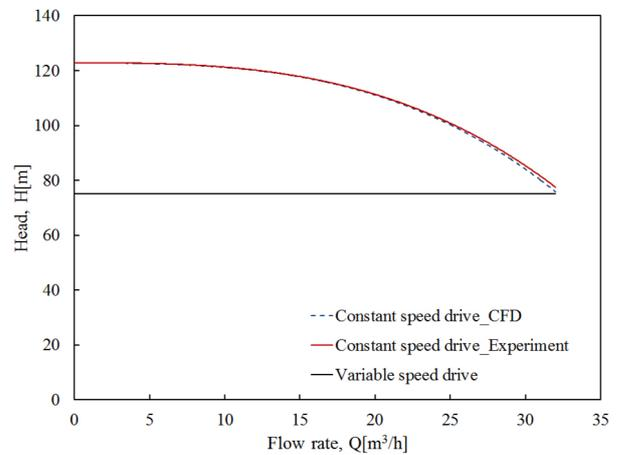
Figure 8:  $H$ - $Q$  curves with constant and variable speed drive
