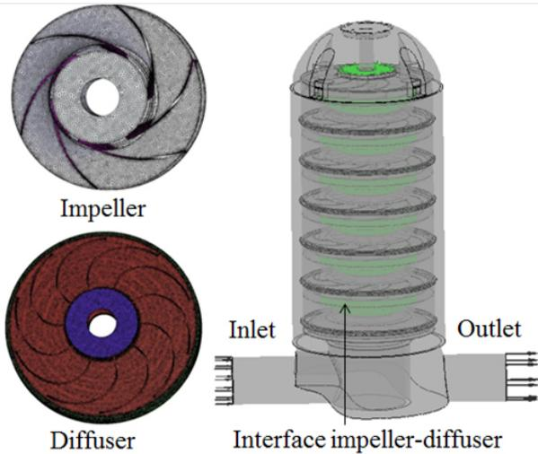
Figure 2: Centrifugal pump model for CFD simulation
