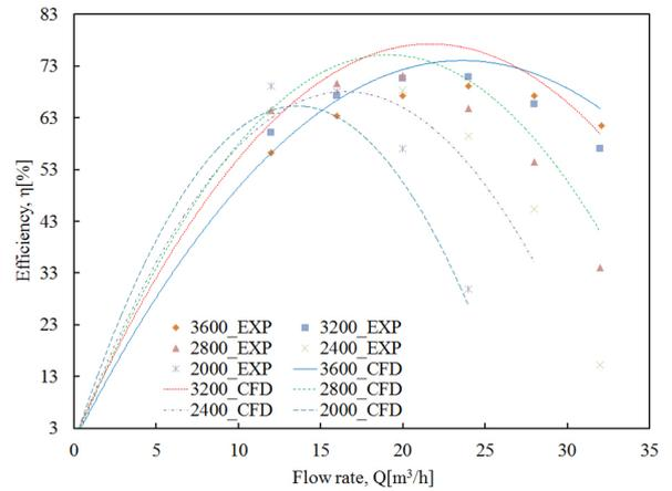
Figure 7:  $\eta$ - $Q$  curves of experiment and CFD simulation
