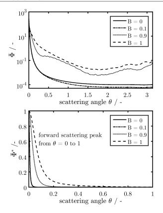
Figure 6: Upper plot: scattering phase function for selected burnout states, log scale. Lower plot: forward scattering peak, normal scale,  $\theta$  ranges from 0 to 1. Note that the plots are normalized to yield 1 for  $\theta = 0$  for comparison
