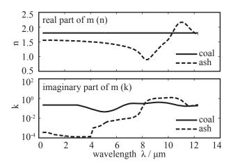
Figure 1: Indices of refraction as applied for coal and ash
