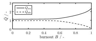
Figure 5: Scattering and absorption efficiencies over burnout
