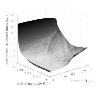
Figure 4: Surface plot of normalized intensity over scattering angle and burnout progress. Intensity is normalized to yield a value of 1 for the sum over  $\theta$  for each burnout state *B*
