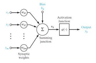
Figure 3: Sketch of the connections to kth neuron in a neural network (Source: [1])
