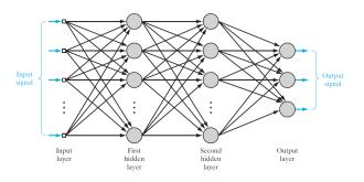
Figure 2: Architectural graph of a multilayer perceptron with two hidden layers. A detailed depiction of a single neuron is shown in Fig. 3 (Source: [1])
