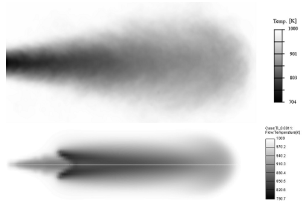
Figure 17: Collation of experimental results [3] and numerical results of temperature in 1.1 ms of injection
