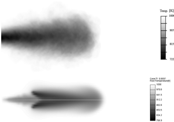
Figure 15: Collation of experimental results [3] and numerical results of temperature in 0.7 ms of injection
