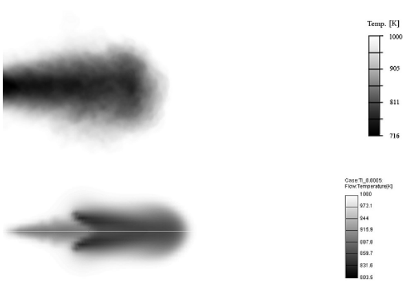
Figure 14: Collation of experimental results [3] and numerical results of temperature in 0.5 ms of injection
