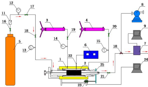
Figure 1: Schematic diagram of the composition of the tri-axial gas seepage experimental system. 1: Coal sample holder; 2: coal samples; 3,4: manual pressure metering pump; 5: high pressure gas tank; 6: thermostat equipment; 7: gas mass flow meter; 8: vacuum pump; 9, 24: computer; 10: three-way valve; 11: pressure-relief valve; 12–15: gauge; 16–21: valve; 22: temperature sensor; 23: displacement sensor; 25: bezel
