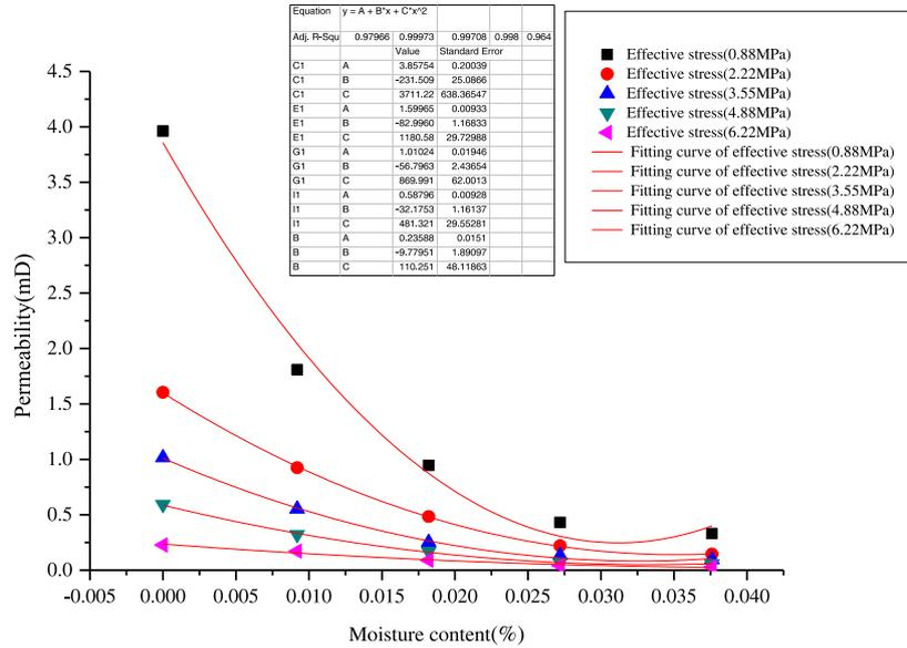
Figure 4: Change curves of permeability under the conditions of different moisture content
