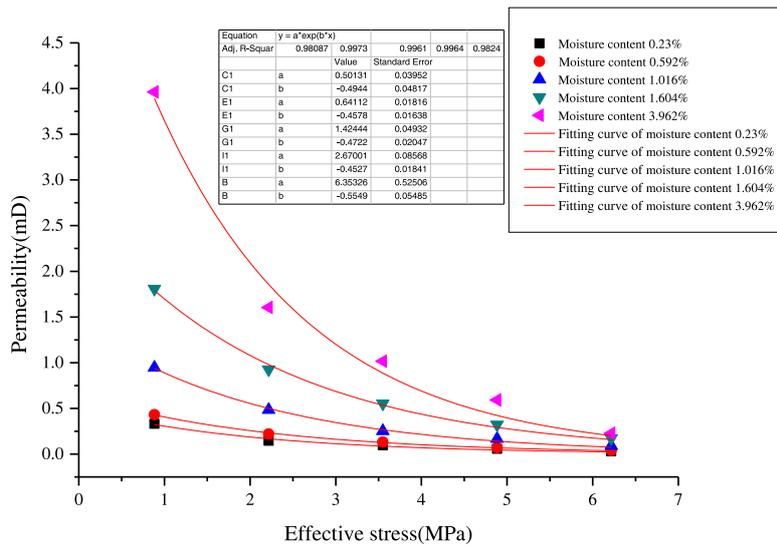
Figure 5: Permeability change curves under different effective stress conditions
