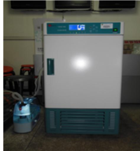
Figure 3: Standard temperature and humidity box
