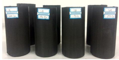
Figure 2: Briquette samples for testing
