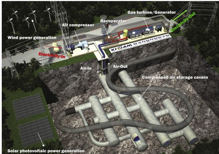
Figure 7: Components of an underground CAES system [43]
