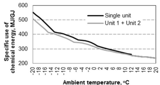
Figure 12: Relation between specific use of chemical energy of fuel and ambient temperature for steam feeding from one and two power units into the heaters (power unit operating at the output of 180 MW)
