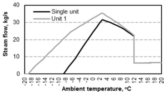
Figure 4: Relation between steam extraction into XC2 heater and ambient temperature for two alternatives of heater feeding (from one and two power units)
