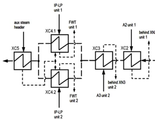
Figure 2: Configuration of heaters with steam bleed from two power units
