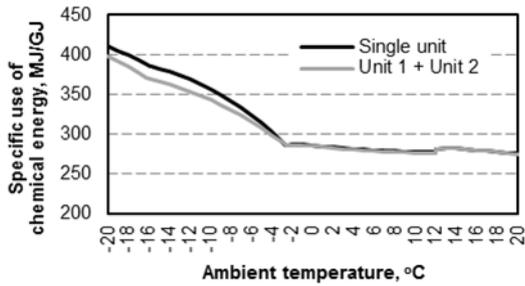
Figure 13: Relation between specific use of chemical energy of fuel and ambient temperature for steam feeding from one and two power units into the heaters (power unit operating at the output of 380 MW)
