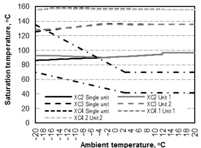
Figure 8: Relation between saturation temperature before XC2, XC3, XC4 (XC4.1, XC4.2) heaters and ambient temperature for steam bleed from one and two units used to feed heaters
