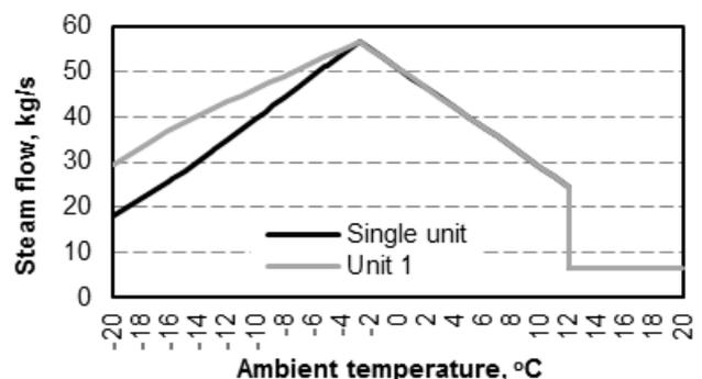
Figure 9: Relation between steam flow into XC2 heater and ambient temperature for heater feeding from one and two power units
