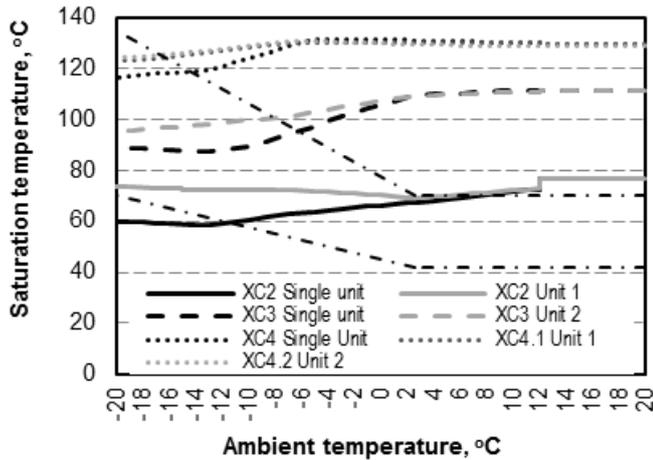
Figure 3: Relation between saturation temperature before XC2, XC3, XC4 (XC4.1, XC4.2) heaters and ambient temperature for steam bled from one and two units used to feed heaters
