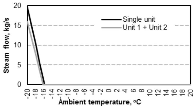
Figure 11: Relation between extraction steam flow into XC4 heater and ambient temperature for heater feeding from one and two power units (for steam extraction from two units the volume extracted into XC4 is made up by the total of flows into XC4.1 and XC4.2)
