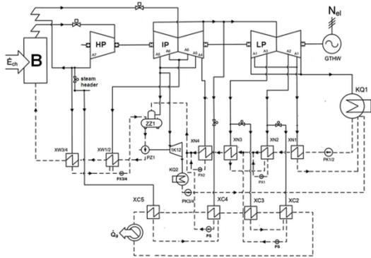
Figure 1: Diagram of a 370 MW unit adapted to cogeneration (B—steam boiler, HP, IP, LP—high-, intermediate- and low-pressure section of the turbine, GTHW—generator, A1, A2, A3, A4, A5, A6, A7—turbine extractions, KQ1, KQ2—condensers in the main and auxiliary turbines, XN1, XN2, XN3, XN4—low-pressure regeneration reheaters, XW1/2, XW3/4—high-pressure regeneration reheaters, XC2, XC3, XC4, XC5—heaters, PZ1—main feedwater pump, PK—condensate pumps, PS—condensate pumps, ZZ1—feedwater tank)
