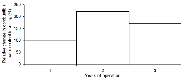
Figure 10: Relative (percentage) change in the combustible content in the slag in consecutive years of biomass co-firing
