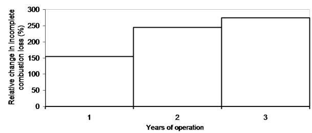
Figure 12: Relative (percentage) change in incomplete combustion loss in consecutive years of biomass co-firing
