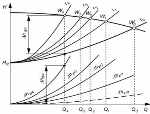
Figure 1: Change in pipeline characteristics  $r = Hp(Q)$  and operating point  $W$  of the pump as a result of the change in the control valve opening level [1]
