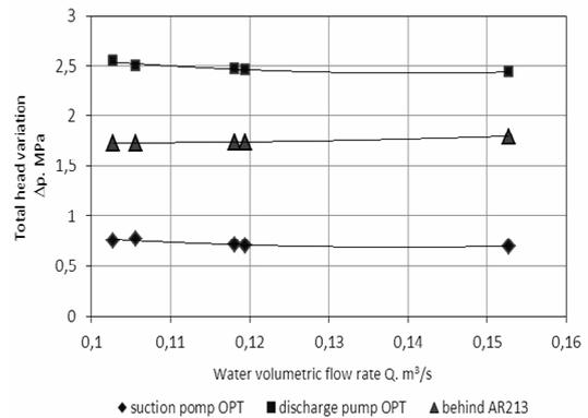
Figure 4: Hydraulic resistance characteristics in the heating water system
