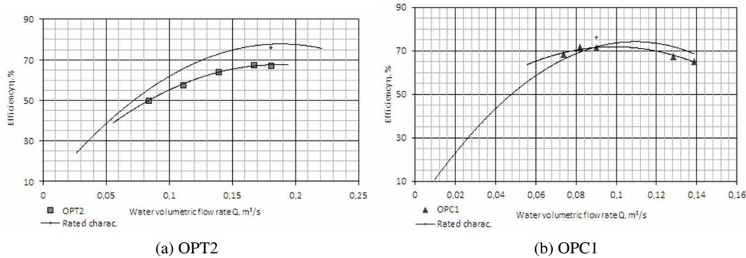
Figure 6: Hot water pump efficiency
