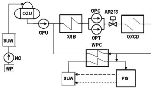
Figure 2: A simplified flow chart of the water closed circuit covering the power plant and the sulfur mine: WP—post-cooling water, NQ—after-cooling water pump, SUW—water treatment station, OZU—water storage tank, OPU—water storage pump, XAB—primary heat exchanger, OPC—hot water pump, OPT—district heating water pump, AR213—control valve, OXCD—peak demand heat exchangers, WPC—recuperative heat exchanger, PG—minefield, SUW—water treatment station
