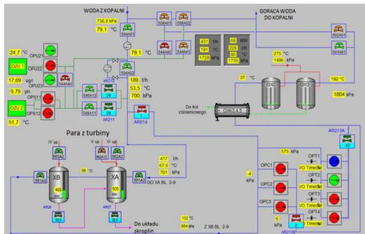
Figure 5: Diagram of system water circuit, main equipment and measurement points
