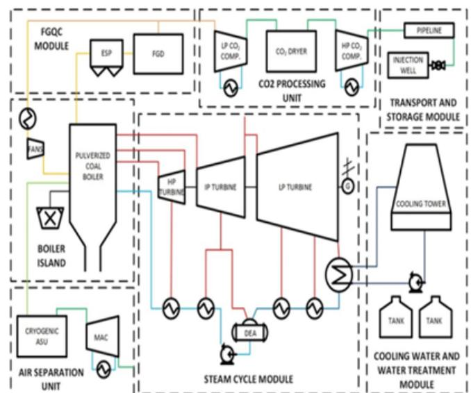
Figure 1: Block-diagram of an integrated OFC power plant with T&S module
