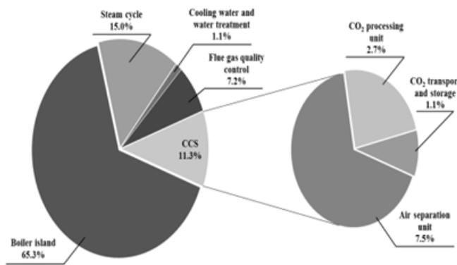
Figure 5: Share of total local exergy losses associated with each technological module of an integrated OFC power plant with CO<sub>2</sub> transport and storage
