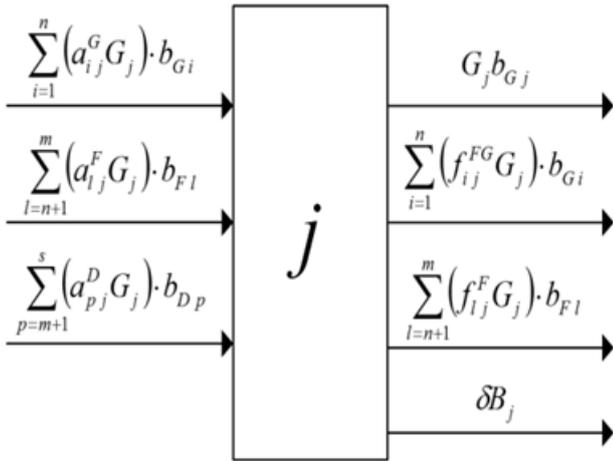
Figure 2: Calculating diagram of local exergy losses
