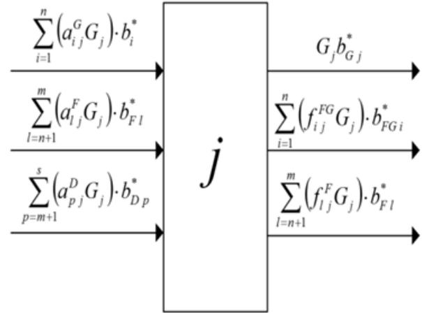
Figure 3: Calculating diagram of cumulative exergy consumption
