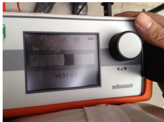
Figure 17: Pinpointing the fixed point; the ESG NT automatically displays the step voltage value and direction
