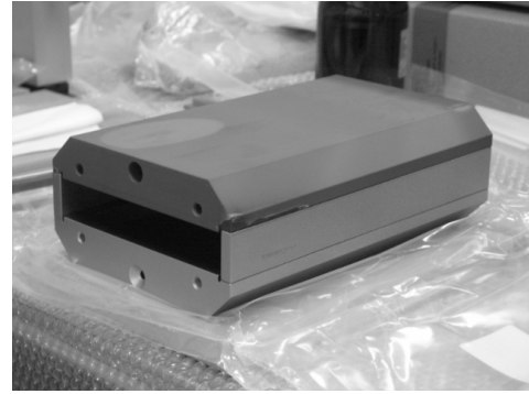
Figure 2: Chamber of Aixtron VP508GFR CVD reactor
