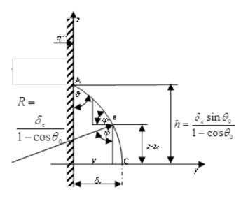
Figure 2: Assumed curvature of the leading edge of the liquid film
