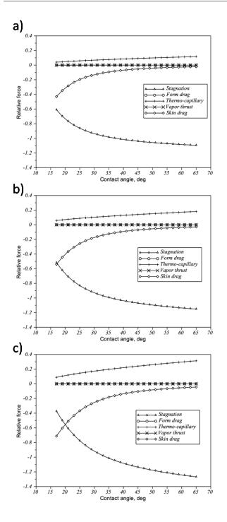
Figure 7: Relative force acting on a dry patch as a function of the contact angle for annular two-phase flow of steamwater mixture; assumed pressure gradient 1700 Pa/m, interfacial shear stress 8.8 Pa, wall heat flux= 1 MW/m<sup>2</sup> at: p = 2 MPa (a), p = 7 MPa (b), p = 12 MPa (c)
