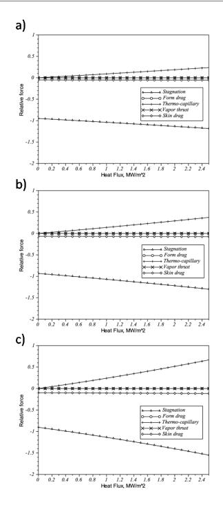
Figure 8: Relative force acting on a dry patch as a function of heat flux for annular two-phase flow of steam-water mixture; assumed pressure gradient 1700 Pa/m, interfacial shear stress 8.8 Pa, contact angle 45°C at: p = 2 MPa (a), p = 7 MPa (b), p = 12 MPa (c)
