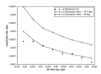
Figure 4: Minimum liquid film flow rate as a function of air flow rate. Comparison of predictions with experimental data [11]
