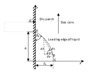
Figure 1: Leading edge of a liquid film upstream of a dry patch
