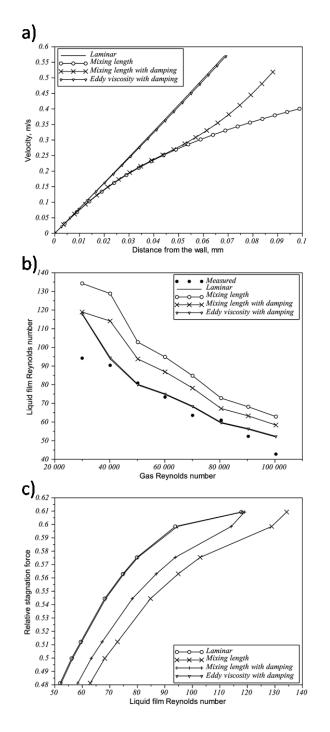
Figure 5: Influence of turbulence models on dry patch rewetting in air-water annular flow in 12.7 mm/31.75 mm annulus at atmospheric pressure and contact angle 24.5°C: velocity profiles in liquid film (a), minimum re-wetting liquid film Reynolds number as a function of gas Reynolds number (b), ratio of stagnation force to surface tension force as a function of the liquid film Reynolds number (c)
