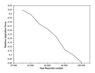
Figure 6: Ratio of stagnation force to surface tension force versus gas Reynolds number for air-water annular flow in 12.7 mm/31.75 mm annulus at atmospheric pressure; contact angle  $24.5^{\circ}$ C
