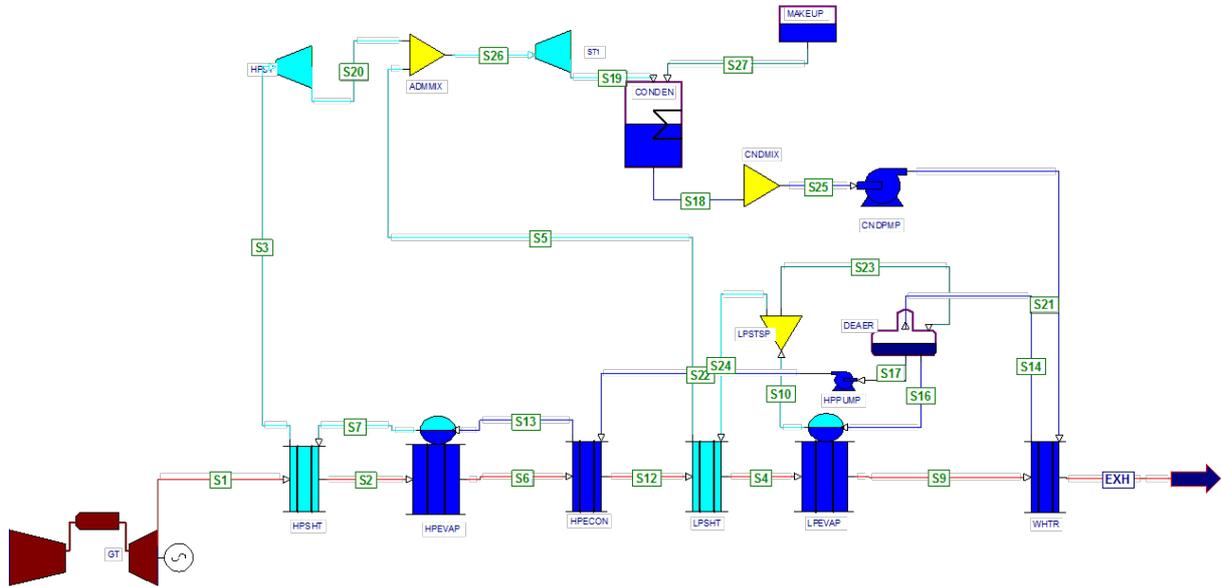
Figure 1: Flowchart of a low-capacity gas-steam system (plant no. 1)
