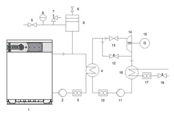
Figure 1: Laboratory installation; 1—gas boiler De Dietrich, 2—oil circulating pump, 3—oil flowmeter, 4—evaporator, 5, 8, 13—ball valve, 6—manometer, 7—safety valve, 9— compensation vessel, 10—mass flowmeter, 11—working fluid pump, 12—throttle valve, 14—expander, 15—alternator, 16— condenser, 17—water meter, 18—throttle valve
