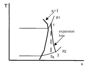
Figure 2: Determination of internal efficiency of expander
