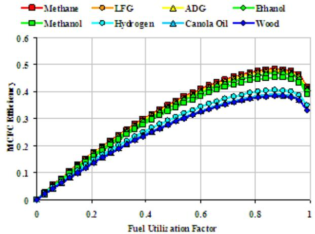
Figure 6: MCFC efficiency vs. fuel utilization factor for various biofuels
