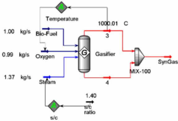
Figure 1: Gasifier model
