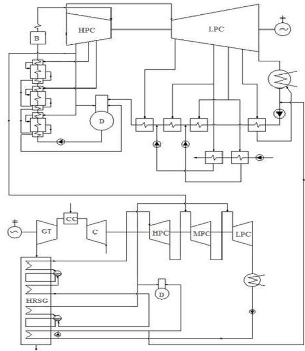
Figure 4: Thermal scheme of PT-80-130 and CCGP with steam turbine-driven compressor joint operation
