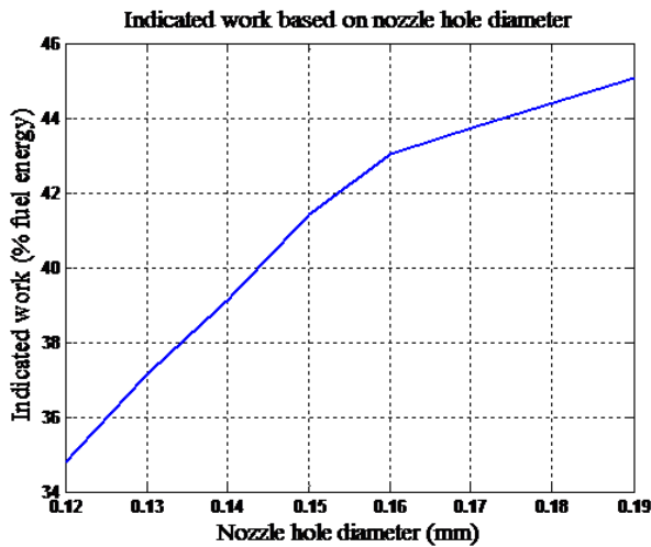
Figure 13: Increase in indicated work by increasing the nozzle hole diameter. This figure shows that increasing the nozzle hole diameter leads to an increase in the indicated work reduced to the fuel energy. Indeed increasing the nozzle hole diameter increases the intensity of combustion, which causes the mean pressure level of gas in the cylinder to rise. This raises the indicated work
