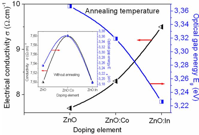
Figure 3: The variation of electrical conductivity  $\sigma$  before and after annealing temperature as a function of the optical band gap energy  $E_g$  for ZnO, ZnO:In and ZnO:Co thin films
