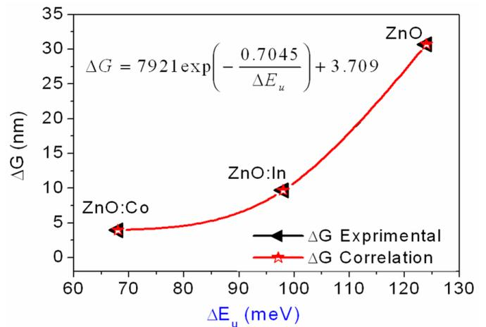
Figure 2: The correlation between the difference in crystallite size ( $\Delta G$ ) with the difference in Urbach energy ( $\Delta E_u$ ) of ZnO, ZnO:In and ZnO:Co thin films
