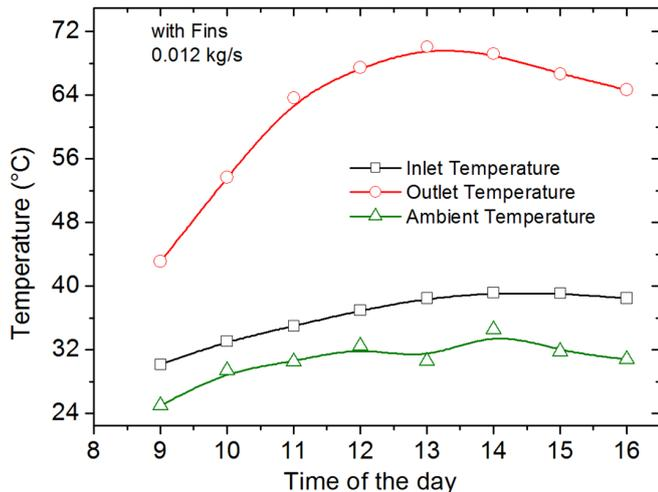
Figure 9: Temperature versus different standard local time during days for single pass solar air heater, at flow rates of 0.012 kg/s, corresponding to the outlet, inlet and ambient temperature of a solar collector with fins
