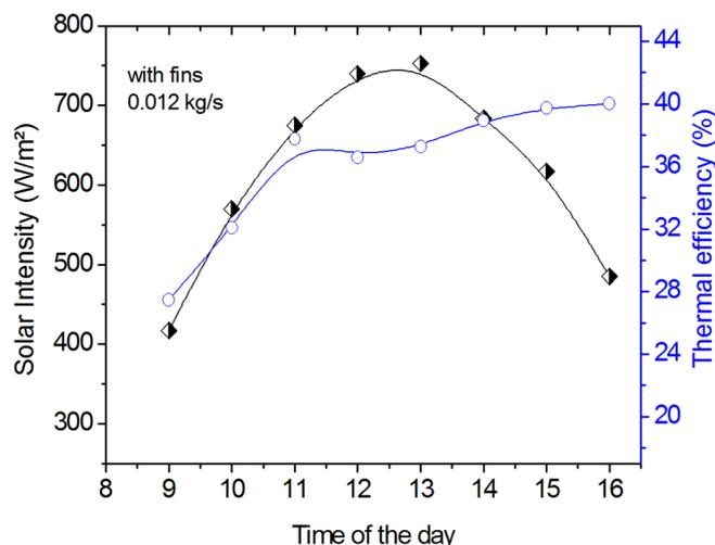
Figure 7: Solar intensity and thermal efficiency versus time of day for a single pass solar air heater, with flow rates at 0.012 kg/s, corresponding to solar collectors with fins
