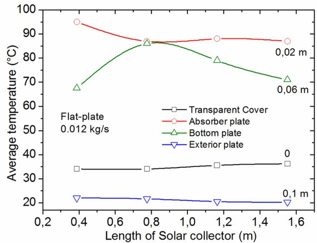
Figure 4: Average temperature along the length of solar collectors versus thickness of panel of between 0 and 0.1 m for single pass solar air heater, at flow rates of 0.012 kg/s, corresponding to the Flat-plate solar collector
