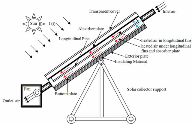
Figure 1: Schematic view of the solar air collector
