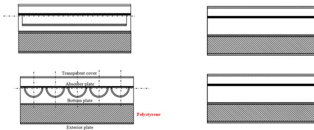
Figure 2: Composition of solar box with and without fins
