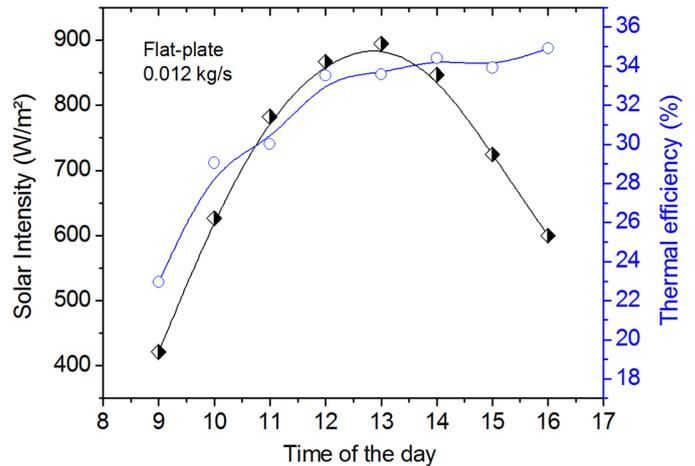
Figure 6: Solar intensity and thermal efficiency versus time of day for a single pass solar air heater, with flow rates at 0.012 kg/s, corresponding to solar collectors without fins
