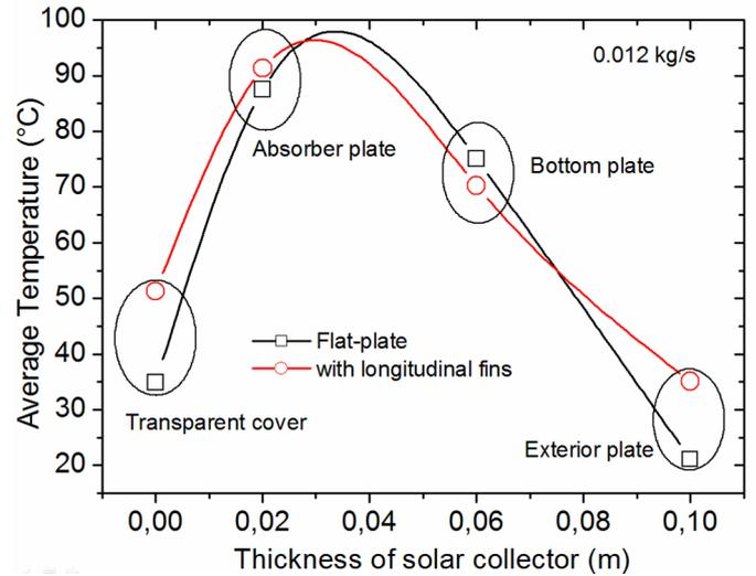
Figure 3: Average temperature in the thickness of a solar collector versus the whole area of the solar collector plates for a single pass solar air heater, with flow rates of 0.012 kg/s, for the solar collectors with and without fins
