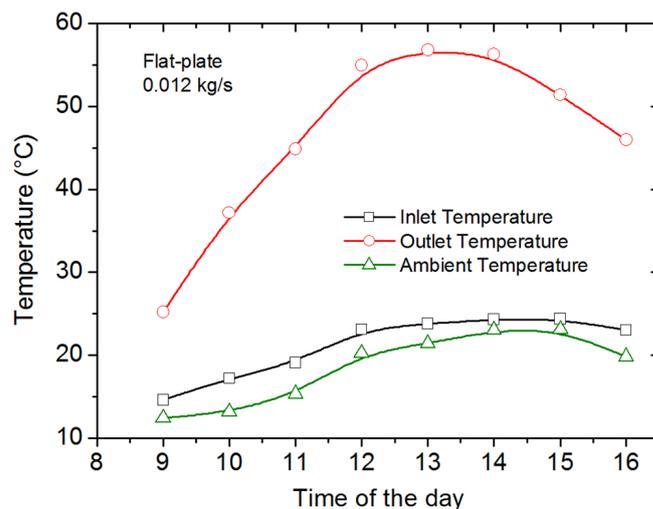
Figure 8: Temperature versus different standard local time during days for single pass solar air heater, of the flow rates at 0.012 kg/s, corresponding to the outlet, inlet and ambient temperature of a solar collector without fins
