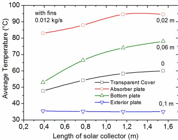
Figure 5: Average temperature along the length of a solar collector versus thickness of panel between 0 and 0.1 m for a single pass solar air heater, with flow rates at 0.012 kg/s, corresponding to solar collectors with longitudinal fins
