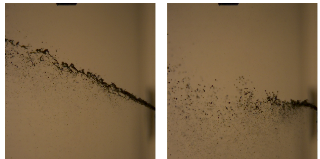
(a) just after start of injection of kerosene without nitrogen flow—8.55 ms
