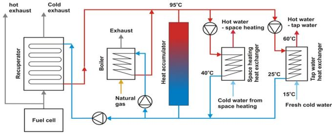
Figure 1: Schematic of the heat recovery system of an SOFC-based micro-CHP
