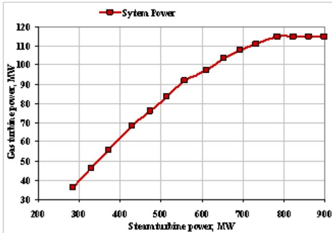
Figure 11: Power achieved by the gas turbine, depending on the power generated by steam turbine
