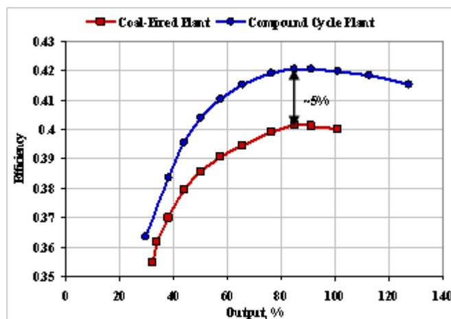
Figure 2: Use of feedwater repowering to increase the efficiency of the steam turbine cycle
