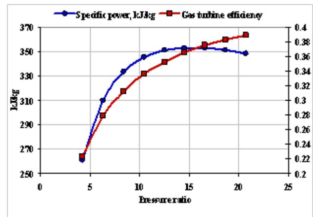
Figure 5: Pressure ratio dependence of specific power and thermal efficiency of the gas turbine
