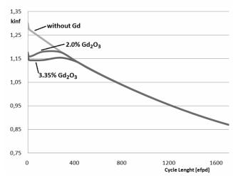
Figure 7: VVER-440 fuel assembly reactivity characteristics of U (without Gd), conventional U/Gd (3.35%) and optimized U/Gd (2.0%)-FAs
