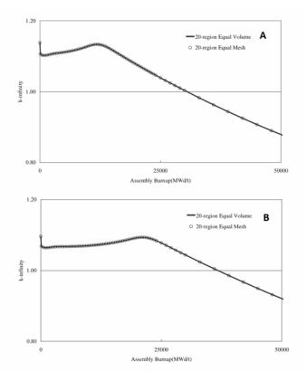
Figure 4: K depending on burnup of PWR fuel assembly  $17 \times 17$  with burnup (A) 48 GWd/tHM and (B) 55 GWd/tHM
