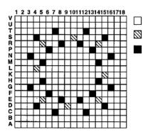
Figure 1: 18x18 U/Gd-fuel assembly with 8 Gd fuel rods [2]
