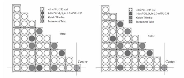
Figure 3: PWR fuel assembly 17×17 with burnup (A) 48 GWd/tHM and (B) 55 GWd/tHM
