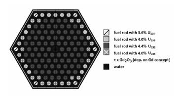
Figure 6: Fuel assembly Gd-2 design, wt. % of GdO depends on Gd concept
