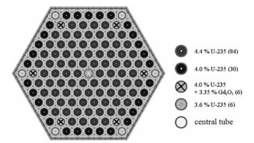
Figure 5: Fuel assembly Gd-2 with enrichment 4.25% (5 year fuel cycle) [4]
