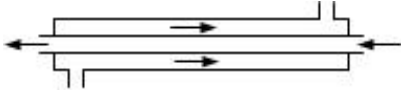
Figure 1: Diagram of a counter-flow heat exchanger with the direction of fluids along the wall
