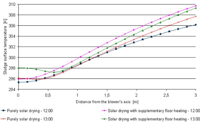
Figure 4: Comparison of the dependency between the sludge surface temperature and the distance from the blower's axis for various hours of the modeled day – for purely solar drying and solar drying with supplementary floor heating
