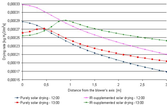
Figure 3: Comparison of the dependency between the drying rate and distance from the blower's axis for various hours of the modeled day – for purely solar drying, and for IR-supplemented solar drying
