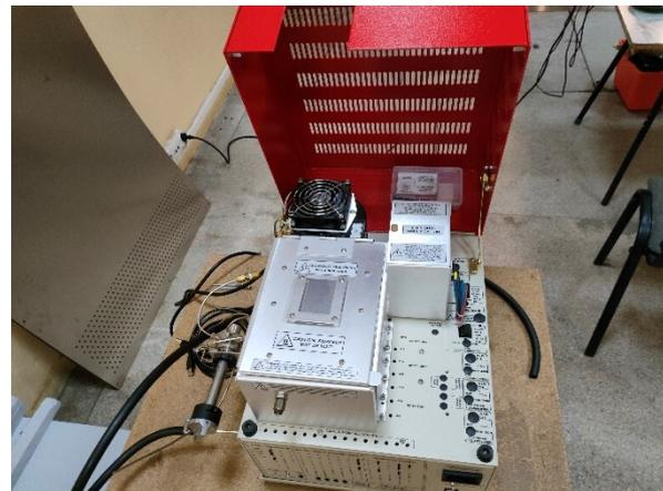
Figure 5: SRI 310C Gas Chromatograph manufactured by SRI INSTRUMENTS, INC.
