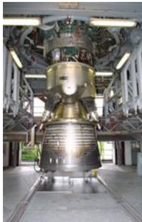
Figure 7. Modern liquid rocket engines with high reliability and reusability- Vulcain 2 engine
