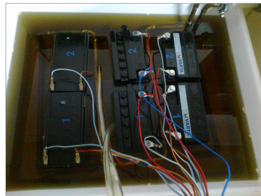
Figure 3: Oil bath setup for the second series of tests
