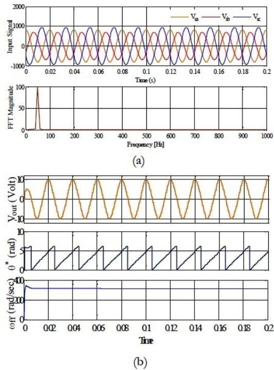
Figure 9: Under voltage unbalance (a) input signal and harmonic spectral (b) transient performance performance.
