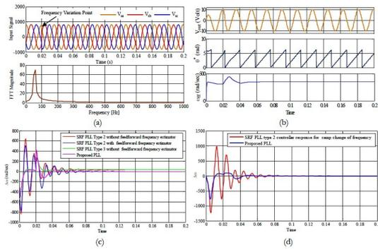
Figure 5: Under Frequency variation (a) Input signal and harmonic spectral (b) transient performance (c) comparative analysis under step change of frequency (d) comparative analysis under ramp change of frequency.
