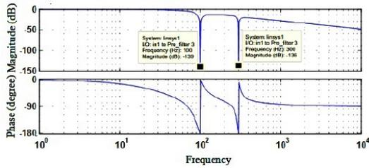
Figure 4: Frequency response Bode plot with selective harmonic filtering.
