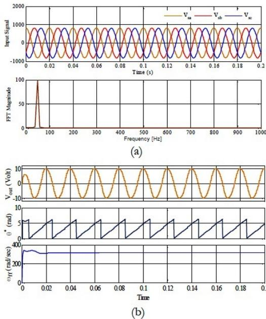
Figure 8: Under unsynchronized phase shift (a) input signal and harmonic spectral (b) transient performance.
