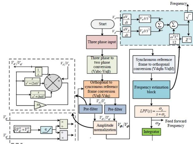
Figure 3: Block diagram of feed-forward frequency estimator.
