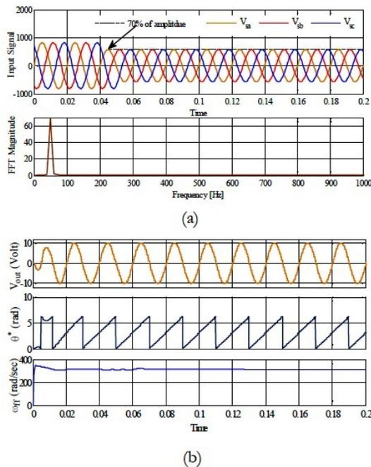
Figure 10: Under voltage unbalance (a) input signal and harmonic spectral (b) transient performance.
