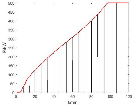
Figure 2: DG output power duration curve
