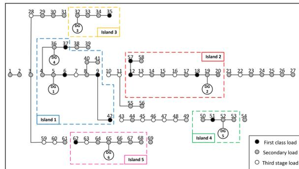
Figure 4: Schematic diagram of primary isolated islands
