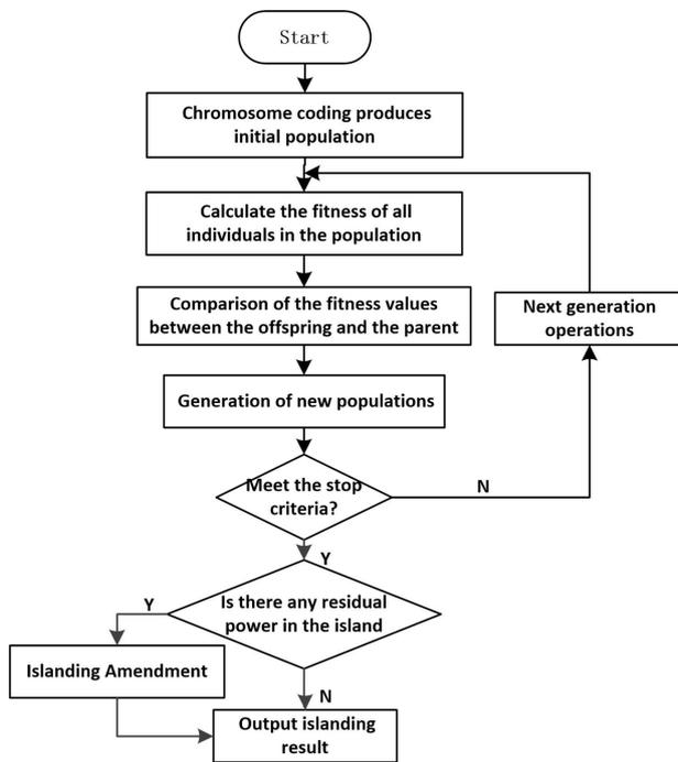
Figure 1: Flow chart of island partition algorithm
