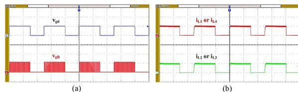
Figure 10: Dimming waveforms at 60% of lamp power (a) Gate control voltages of  $S_d$  and  $S_B$  (b) Current waveforms of all four lamps ( $i_{L1}$ ,  $i_{L2}$ ,  $i_{L3}$ ,  $i_{L4}$ : 1 A/div; time: 4 ms/div)
