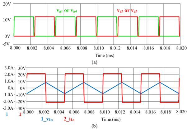
Figure 5: Simulation waveforms (a) Gate voltages of switches in full bridge. (b) Voltage and current in  $L_s$ .
