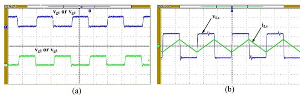
Figure 6: Experimental waveforms (a) Gate voltages of switches in full bridge ( $v_{g1}, v_{g2}, v_{g3}, v_{g4}$ : 14 V/div; time: 2  $\mu$ s/div). (b) Voltage and current in  $L_s$  ( $v_{Ls}$ : 14 V/div;  $i_{Ls}$ : 1 A/div; time: 2  $\mu$ s/div).
