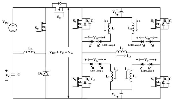
Figure 1: Proposed full bridge LED driver circuit
