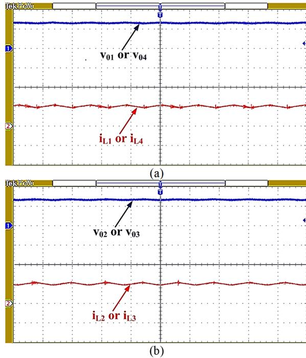
Figure 8: Experimental waveforms (a)  $V_{01}$  voltage and current waveforms at full illumination in LED lamp-1 and lamp-4. (b) Voltage and current waveforms at full illumination in LED lamp-2 and lamp-3 ( $v_{01}$ ,  $v_{02}$ ,  $v_{03}$ ,  $v_{04}$ : 25 V/div;  $i_{L1}$ ,  $i_{L2}$ ,  $i_{L3}$ ,  $i_{L4}$ : 1 A/div; time: 8  $\mu$ s/div).
