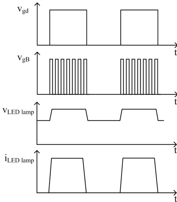
Figure 4: Waveforms under dimming control
