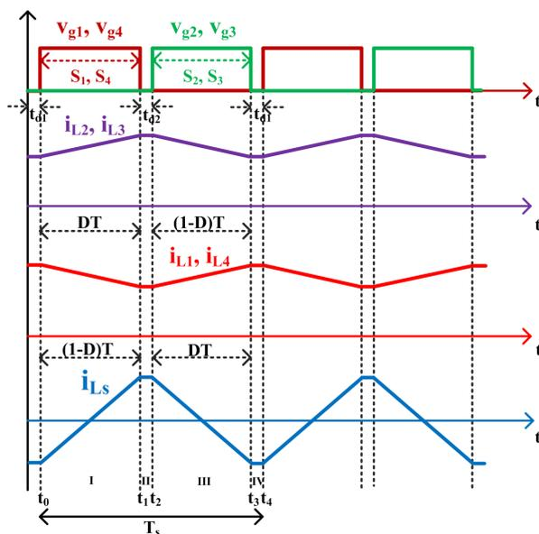
Figure 2: Operating waveforms of proposed LED driver circuit
