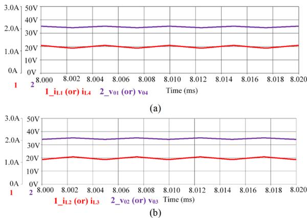
Figure 7: Simulation waveforms (a)  $V_{01}$  voltage and current waveforms at full illumination in LED lamp-1 and lamp-4. (b) Voltage and current waveforms at full illumination in LED lamp-2 and lamp-3.
