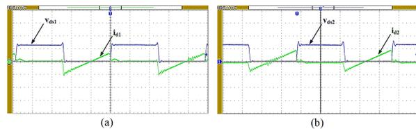
Figure 9: Experimental switching waveforms (a) Voltage and current in Switch  $S_1$  (b) Voltage and current in Switch  $S_2$  ( $v_{ds1}$ ,  $v_{ds2}$ : 14 V/div;  $i_{d1}$ ,  $i_{d2}$ : 1 A/div; time: 1  $\mu$ s/div).
