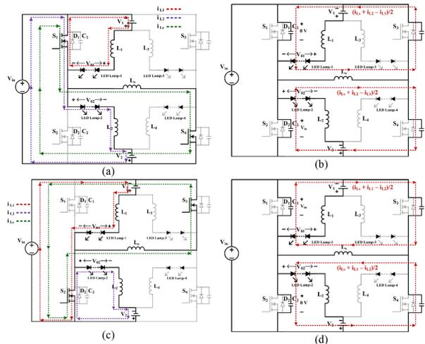
Figure 3: Equivalent circuits of proposed LED driver. (a) Mode-I. (b) Mode-II. (c) Mode-III. (d) Mode-IV.
