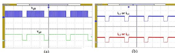
Figure 11: Dimming waveforms at 80% of lamp power (a) Gate control voltages of  $S_d$  and  $S_B$  (b) Current waveforms of all four lamps ( $i_{L1}$ ,  $i_{L2}$ ,  $i_{L3}$ ,  $i_{L4}$ : 1 A/div; time: 4 ms/div)
