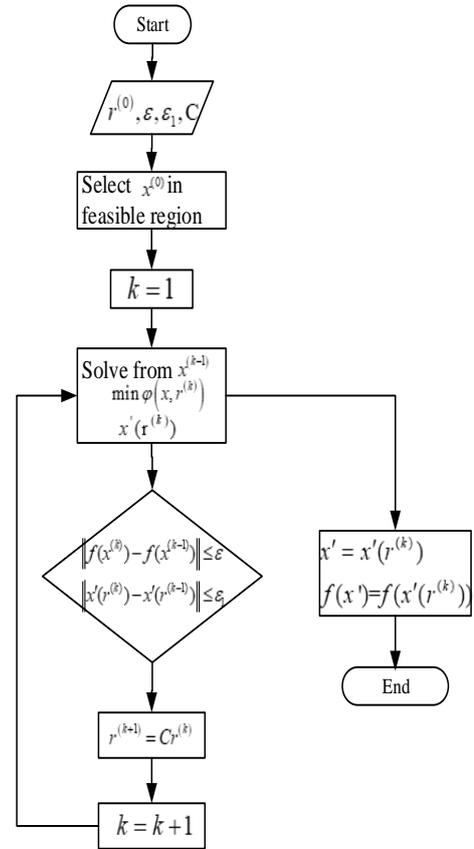
Figure 1: Calculation program diagram of the interior point method
