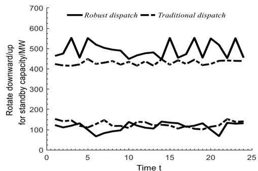
Figure 6: Reserve capacity comparison between traditional and robust dispatch methods
