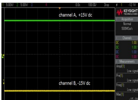
Figure 18: output waveform of AC to DC converter
