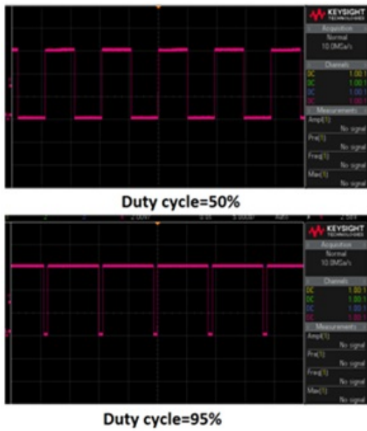
Figure 21: PWM output waveform with different duty cycle
