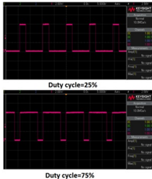
Figure 20: This is a PWM output waveform with different duty cycle caption
