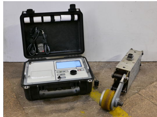
Figure 3: MRT testing head with a defectograph
