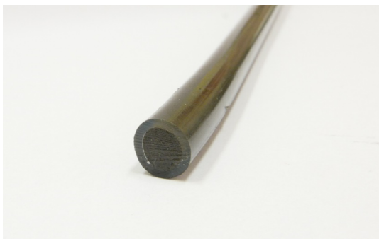
Figure 5: Model of the composite core containing FeSi powder
