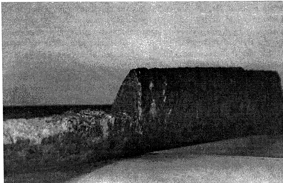
Fig.2. A characteristic shape of the deposit on a tube surface (from a steam superheater of the boiler from Laziska Power Plant)
