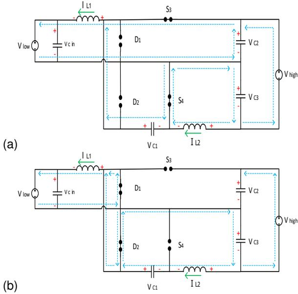
Figure 5: Operational modes of the proposed converter in buck state a) first level; b) second level
