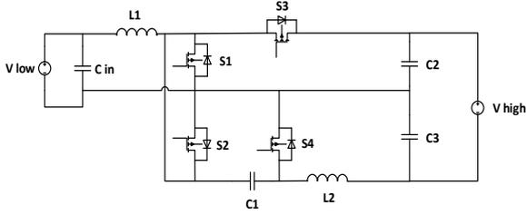
Figure 1: The proposed bidirectional DC-DC Converter
