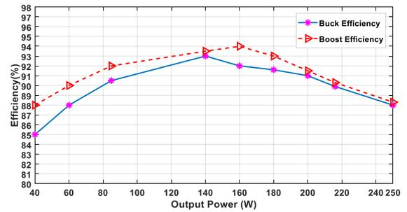
Figure 10: The efficiency curves in buck and boost states
