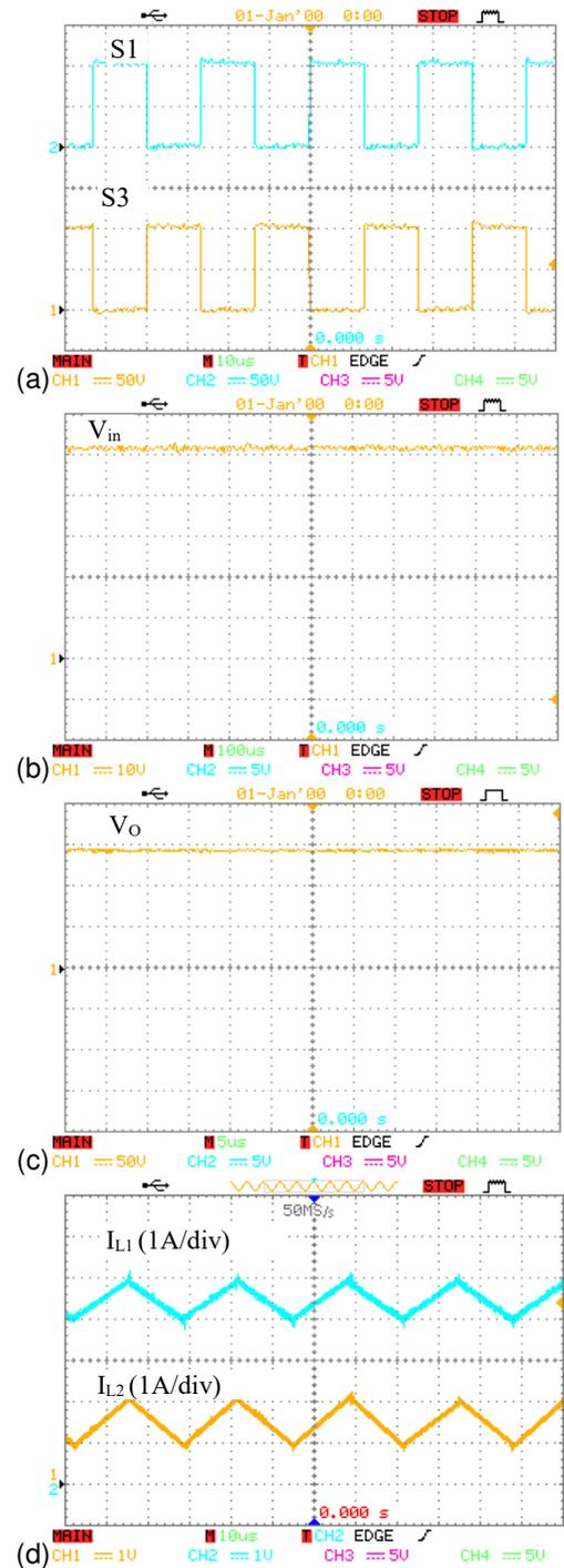
Figure 8: Experimental results of the proposed converter in step-up state. (a) voltage of  $S_1$  and  $S_3$ , (b) input voltage, (c) output voltage and (d) Inductors current  $L_1$  and  $L_2$
