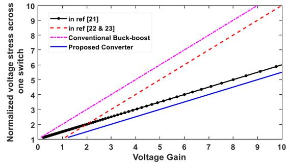
Figure 3: Voltage stress curve for the different voltage gain of the proposed converter and other converters
