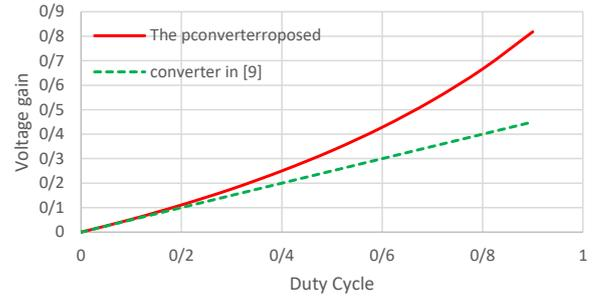
Figure 6: The gain curve of the proposed converter
