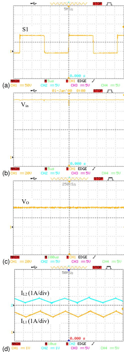
Figure 9: Experimental results of the proposed converter in step-down state. (a) voltage of the S1, (b) input voltage, (c) output voltage and (d) Inductors current  $L_1$  and  $L_2$
