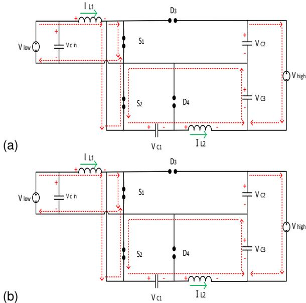
Figure 2: Operational modes of the proposed converter in boost state a) first mode; b) second mode
