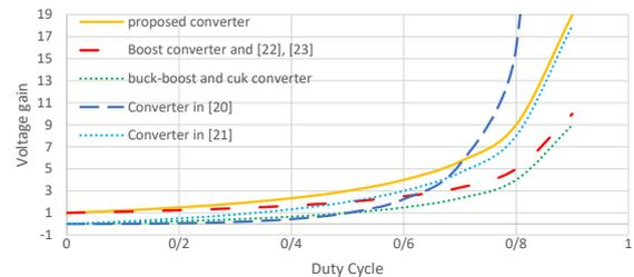
Figure 4: Voltage gain curve of the proposed converter and other converters for different duty cycles.
