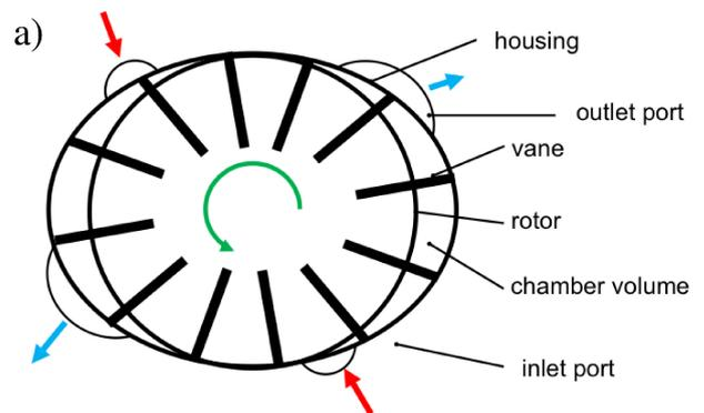
Figure 3: Schematic of the dual chamber radial expander [6]
