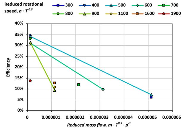
Figure 16: Efficiency curves for expander operated on carbon dioxide as functions of reduced mass flow,  $\frac{\dot{m} \cdot \sqrt{T}}{p}$  for various reduced rotational speeds,  $\frac{n}{\sqrt{T}}$
