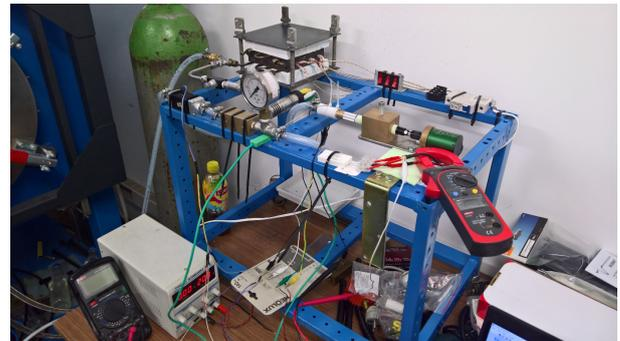
Figure 12: The test stand for characterization of micro rotary sliding vane expander operated on CO<sub>2</sub>
