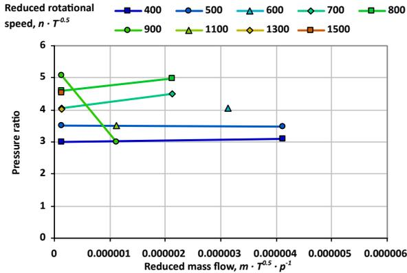
Figure 13: The expander operated on air pressure ratio as a function of reduced mass flow,  $\frac{\dot{m} \cdot \sqrt{T}}{p}$  for various reduced rotational speeds,  $\frac{n}{\sqrt{T}}$
