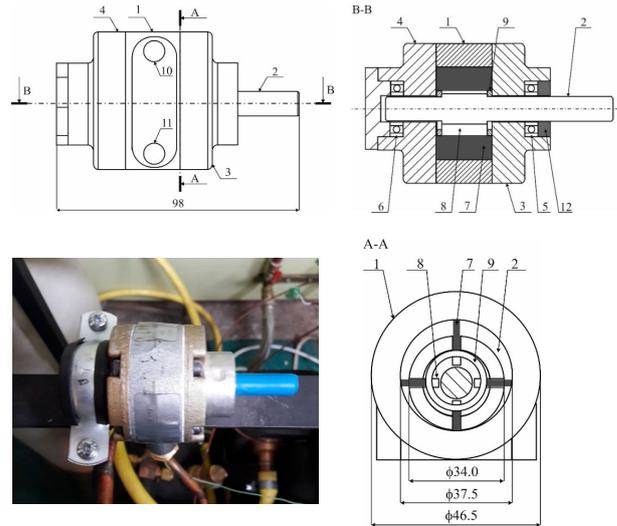
Figure 7: A general view and simplified construction scheme of the expander [9]
