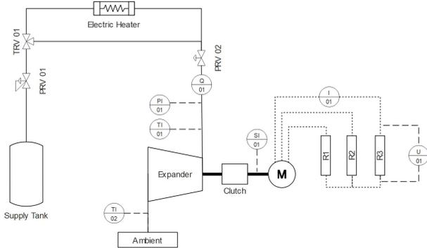
Figure 9: Simplified schematic of the laboratory stand for characterization of rotary sliding vane expander
