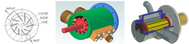
Figure 8: A cross-section of the expander used for  $\mu$ CHP plant [10]
