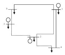
Figure 5: Garver's Test System [18]
