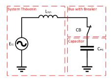
Figure 1: Capacitor Switching Model
