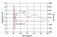
Figure 4: Voltage due to capacitors for back-to-back switching [17]
