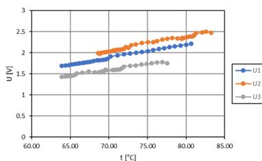
Figure 4: Voltage characteristics of Peltier modules as a function of the temperature difference (U1 - TEC1-12715, U2 - TEC1-12710, U3 - TEC1-12708)
