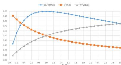
Figure 1: Dimensionless functions of the Peltier thermogenerator's operating parameters
