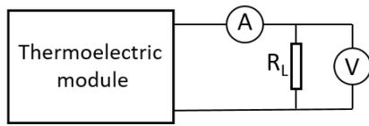
Figure 3: Schematic diagram of the measurement electric circuit
