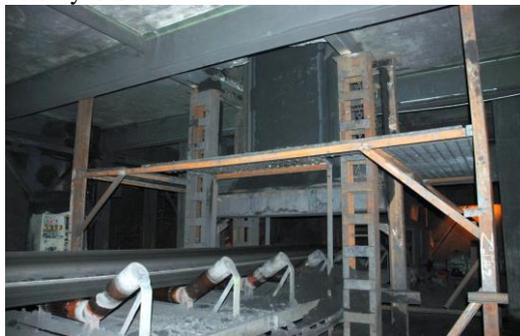
Figure 10. Support for Gravity take-up Arrangement
