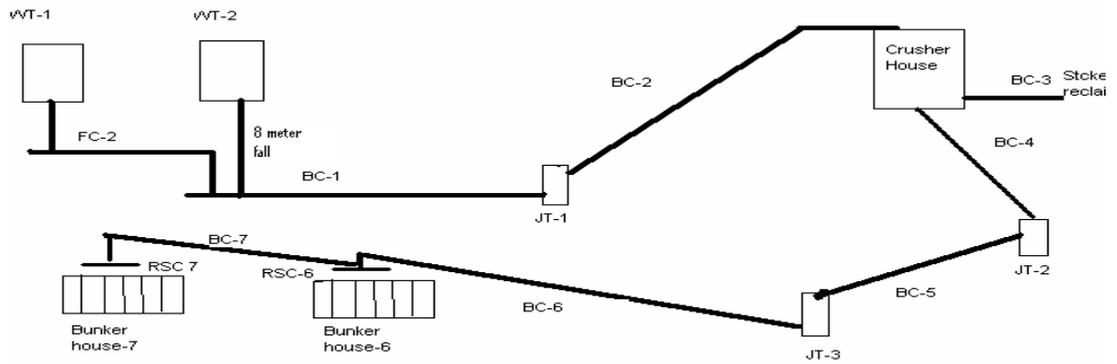
Figure 5: Single stream conveyor system at new NP TPS
