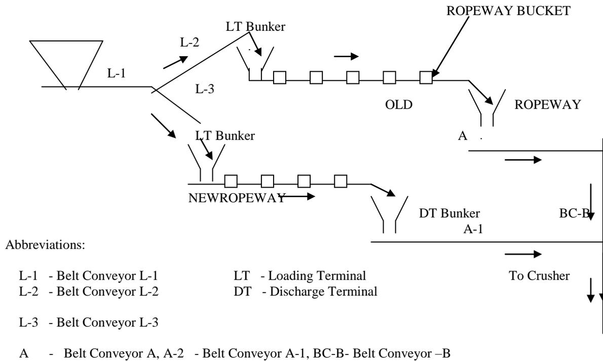
Figure 2: Line diagram of ropeway system
