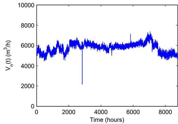
Figure 5: Hourly demand curve of industrial customer (flow at standard conditions of 101.325 kPa and 273.15 K)
