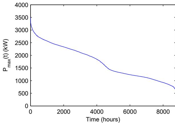
Figure 4: Duration curve of power output (theoretical limit value) in Case study I
