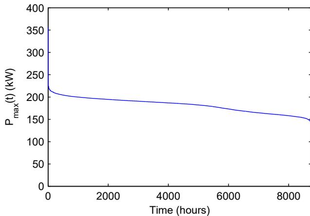
Figure 8: Duration curve of power output in Case study II
