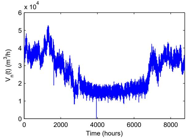
Figure 1: Hourly demand curve in a municipal area (flow at standard conditions of 101.325 kPa and 273.15 K)
