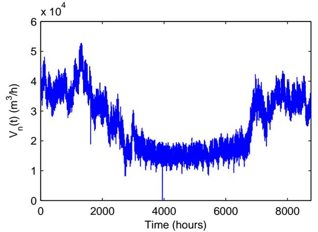
Figure 1: Hourly demand curve in municipal area (flow at standard conditions of 101.325 kPa and 273.15 K).
