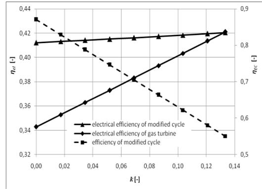
Fig.5. Electrical efficiency  $\eta_{el}$  and the efficiency of the entire power plant  $\eta_{EC}$  depending on  $k$ , with  $\dot{m}_f = \text{const.}$
