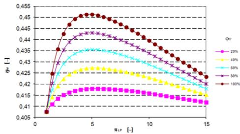
Fig.7. System electric efficiency  $\eta_{el}$  versus compressor low-pressure part compression ratio and relative air humidity  $\phi$  after humidification, with  $\dot{m}_f = const.$
