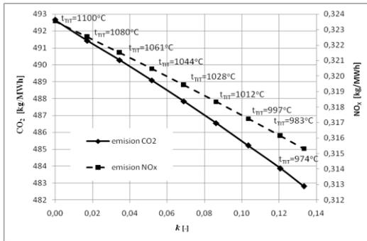
Fig.4. Relationships of the emission of carbon dioxide  $\text{CO}_2$  and nitrogen oxides  $\text{NO}_x$ , and temperature before the gas turbine  $t_{TTR}$  depending on  $k$ , with  $\dot{m}_f = \text{const.}$
