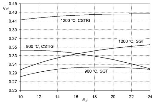
Fig.6. Dependence of the electrical efficiency  $\eta_{el}$  of CSTIG ( $k = 0.04$ ) and simple gas turbine SGT ( $k = 0.0$ ) from compressor pressure ratio  $\pi_c$  for the turbine inlet temperature  $t_{III} = 900$  °C and 1200 °C.
