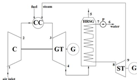
Fig. 1. Scheme of gas-steam cycle with possibility of transition to the STIG, (GT - gas turbine, C - compressor, CC - combustion chamber, G - generator, HRSG - heat recovery steam generator, ST - steam turbine, P - pump, CON - condenser, WH - heat exchanger) [6].
