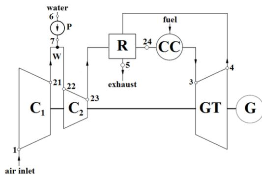
Fig.3. Scheme of system with regeneration and interstage cooling in compressor by using water injection (C1, C2 - low- and-high pressure compressor, R – regenerative heat exchanger, CC – combustion chamber, GT – gas turbine, G – generator, W - water injection, P - pump).
