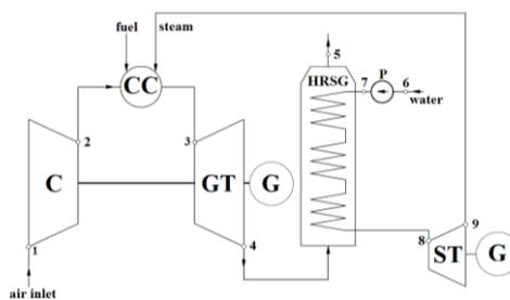
Fig. 2. Scheme of CSTIG system (GT – gas turbine, C – compressor, CC – combustion chamber, G – generator, HRSG – heat recovery steam generator, ST – steam turbine, P – pump).
