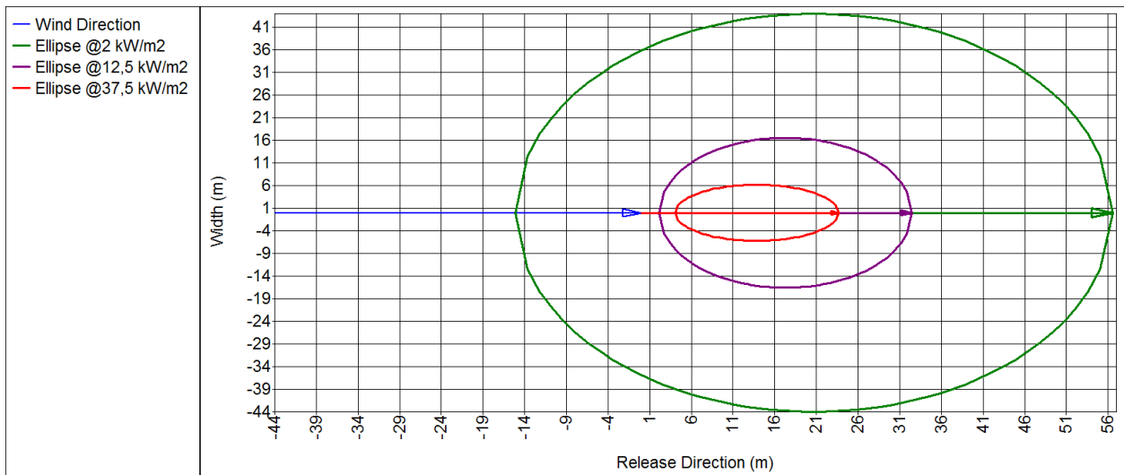
Figure 4: Hazard zone ranges (horizontal outflow)
