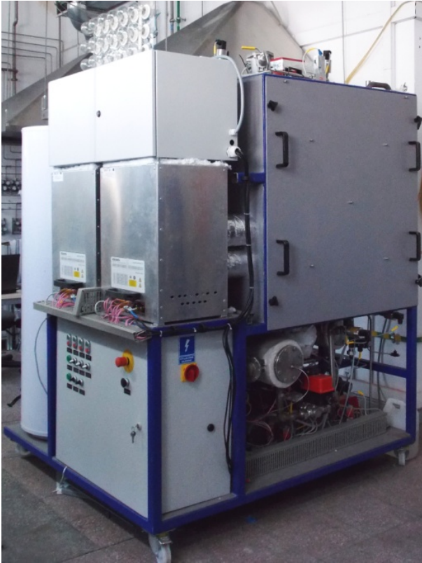
Figure 3: Micro-combined heat and power unit with solid oxide fuel cell stacks—view showing the high temperature chamber
