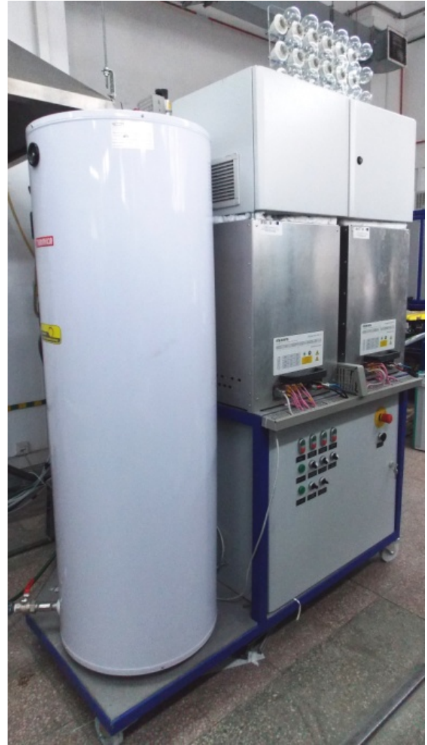
Figure 2: Micro-combined heat and power unit with solid oxide fuel cell stacks—view showing the 140 l hot water storage tank
